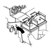
Place the suction end of the NovaPrime over the jet area of the cartridge.
